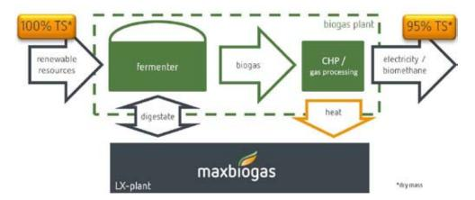
The easiest application is the pre-treatment of biogas digestate. The solid parts of the digestate are mainly composed of cellulose und hemicelluloses which were not available for biogas production. The maxbiogas LX-plant pre-treats the digestate in such a way that it is transformed almost completely into biogas in the biogas plant fermenter. The energy used by the maxbiogas process is supplied by the power generation or by the gas purification of the biogas plant.
